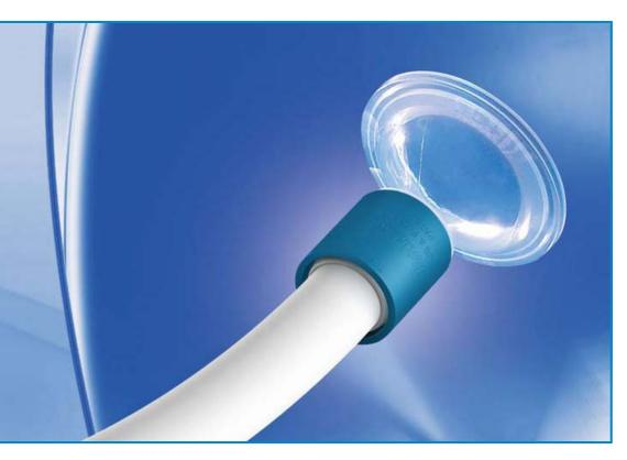
When it comes to retaining flexible tubing and hose onto barbed fittings, the BarbLock<sup>®</sup> retainer is the most advanced product currently available. BarbLock<sup>®</sup> is the only retainer with a full 360-degree radial crimp behind the barb and 360 degrees of compression directly over the barb's ridge, a design that solves inherent leak path problems in demanding fluid transfer applications.
