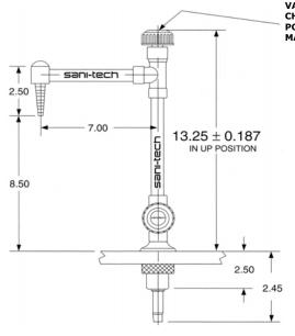
VACUUM BREAKER WITH CHECK VALVE, POSITIVE POSITION INDICATOR, MANUAL OVERRIDE
