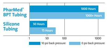
The performance of tubing in peristaltic pumping applications is affected by the conditions of use and equipment utilized, along with size and wall thickness of the tubing tested. The data above is presented for information only and should not be utilized for specification purposes.
