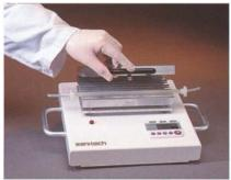
Place the tubing into the heater block.
