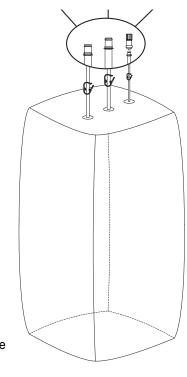
With C-Flex Clear 374 Tubing, MPX Insert Fittings (Male), Female Luer®Lock with Needle-Free Sampling Port
