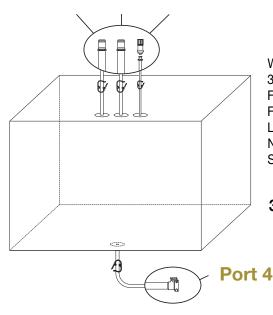
With C-Flex® Clear 374 Tubing, MPX Fittings (Male & Female), Female Luer®Lock with Needle-Free Sampling Port
