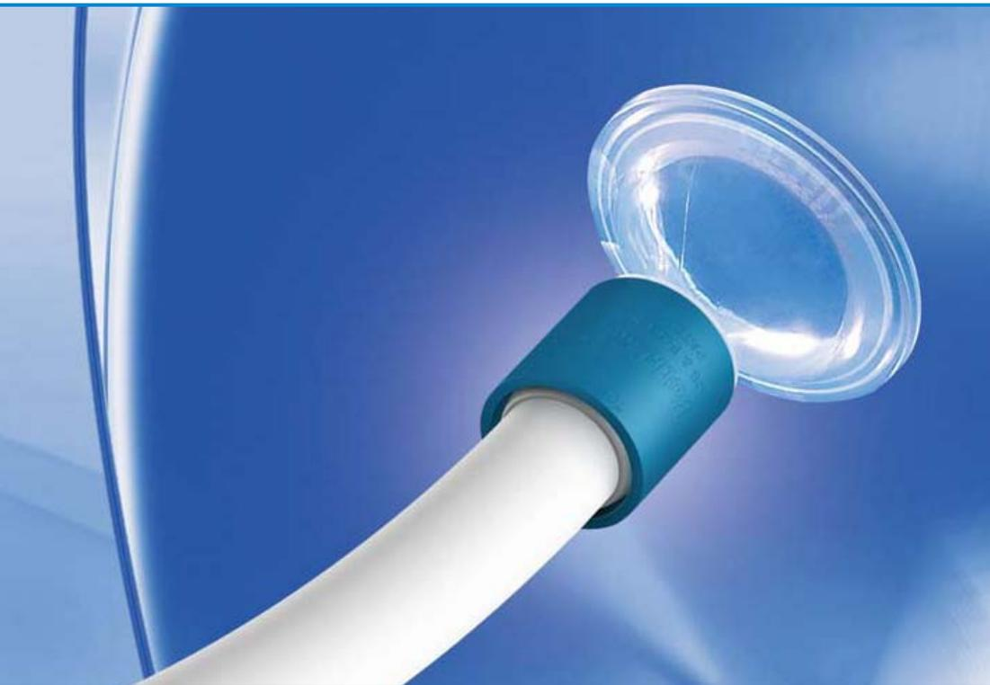
When it comes to retaining flexible tubing and hose onto barbed fittings, the BarbLock® retainer is the most advanced product currently available. BarbLock® is the only retainer with a full 360-degree radial crimp behind the barb and 360 degrees of compression directly over the barb's ridge, a design that solves inherent leak path problems in demanding fluid transfer applications.
