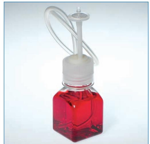
Single 60mL sampling bottle showing Bio-Simplex<sup>™</sup> Closure Assembly with an EZ Top<sup>®</sup> container closure.
