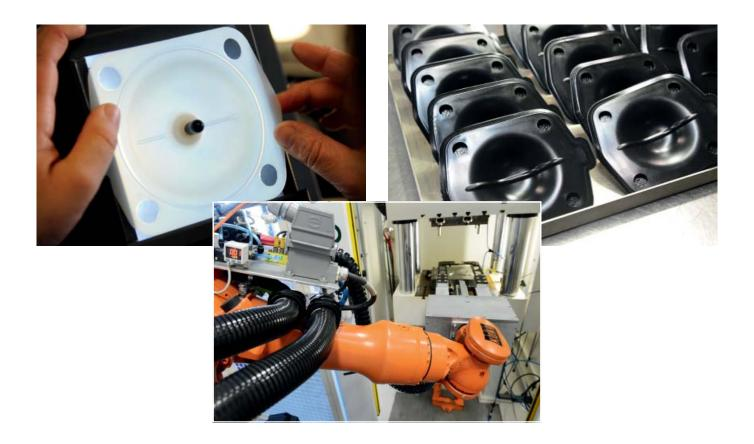
Manufacture of elastomer parts using vacuum injection and compression moulding
