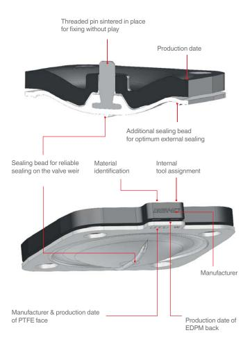
The GEMÜ PTFE/EPDM diaphragms comprise a PTFE face and an EPDM back. These two components are either firmly (Code 5A/52) or flexibly (Code 5E) combined with each other.
