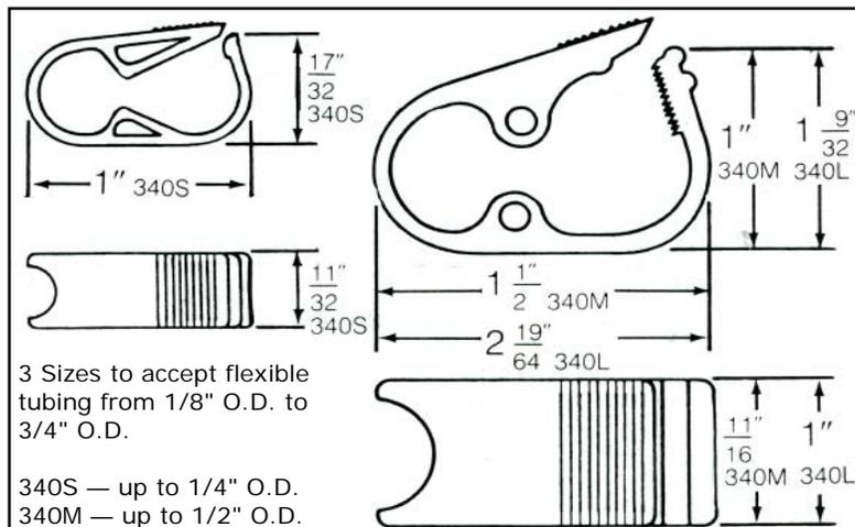
Pinch Clamp 340M and 340L feature 12 position control with ratchet to throttle flow evenly to complete closure.
