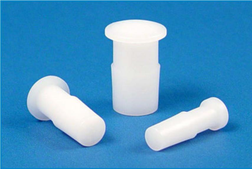
Sani-Plugs provide a superior seal to tubing through a single-barb construction. Tubing clamps secure to the fittings behind the barbed area, which limits the risk of tubing being cut from a sharp, barbed edge and provides for attachment to a smooth surface.
