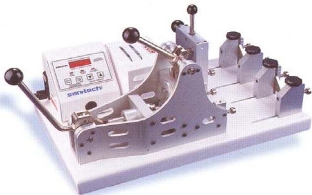
**Sani-Tech Flange Formers** allow complete portability to produce sanitary Tri-Clamp® flanges at any location in the plant. These components complement or replace stainless steel, glass or industrial plastic piping systems. Sani-Pro Rigid sanitary tubing features smooth bore construction, assuring smooth product flow and no crevices.
