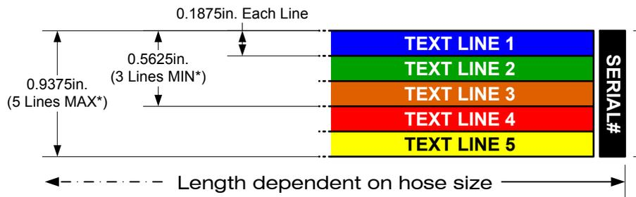
**New – Assembly Serial # placement.**
