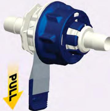
Twist the blue lock ring clockwise until audible "Colder Click." Alignment of the lock ring rib with the body's arrow indicator confirms final connection.
