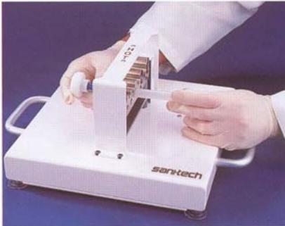
Place the tubing end and the sanitary ferrule on the heater head.
