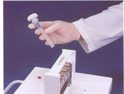
Position the mandrel and apply pressure to create fusion.
