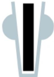
The Envelope seal construction provides **inconsistent** results between the two materials. It will also creep, cold flow and leak over time.
