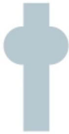
A Solid PTFE Type I seal is guaranteed to fail in SIP conditions. They will creep, cold flow and leak at  $\Delta T$ .
