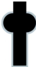
The PTFE grafted elastomer in a Tuf-Flex seal will maintain I.D. without re-torquing or leaking.
