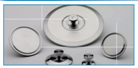
The i-cap, engineered and patented by I-4, Inc., makes removal of end caps easier and safer for both the user and equipment. The i-cap's unique I shape fits into the pronged end of any standard Tri-Clamp® clamp. Just hook the clamp onto the i-Cap and it pops off easily without risk of injury or damage to the end cap face or attached equipment.
